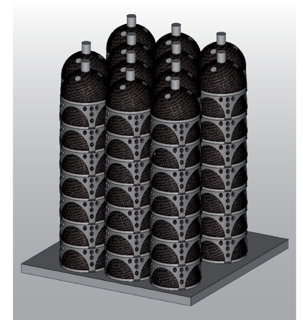
STL file, tower stacking of acetabular cups for maximum productivity
